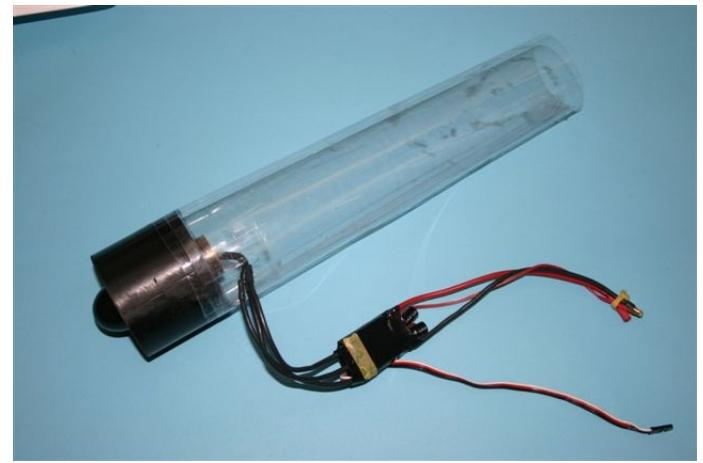
Read the installation instruction from your fan-unit first. Install motor and ESC first. You can either install the ESC inside the thrust tube or outside. We recommend to place the ESC behind the motor inside the thrust tube.
