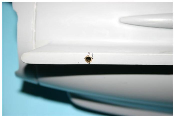
Mark the position for the Pivot-tube ( 2 4 mm brass tubes one for each side) 40 mm from the end of the fuselage fairing. Drill the hole in the middle. Drill a little oversized hole in the middle at the marked location. We recommend a 5 mm hole. Wait before you glue the pivot tube in place.
