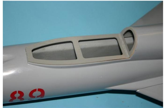
Get the canopy bottom , front and the back plate , place on the fuselage . secure the bottom plate with some tape. Now glue the back plate to plywood canopy bottom. Paint the canopy frame grey.
