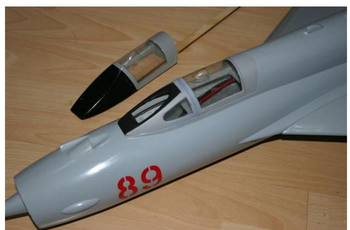
When you have finished the painting u can cut out either the front window or all 3 front window. This will act as an extra intake. You can also or instead of, cut cheater-holes under de fuselage Under the wing root on both sides 1 round hole 20 mm diameter.
