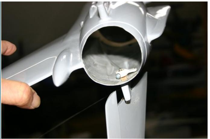
Before you glue the Pivot tube in the fuselage with 5 minute epoxy put tape around the root of the Elevon. And also put tape over the fuselage side. Glue one pivot tube at the time, and check the alignment. Notice the control-horn top hole is trimmed off. The horn is pointing down.
