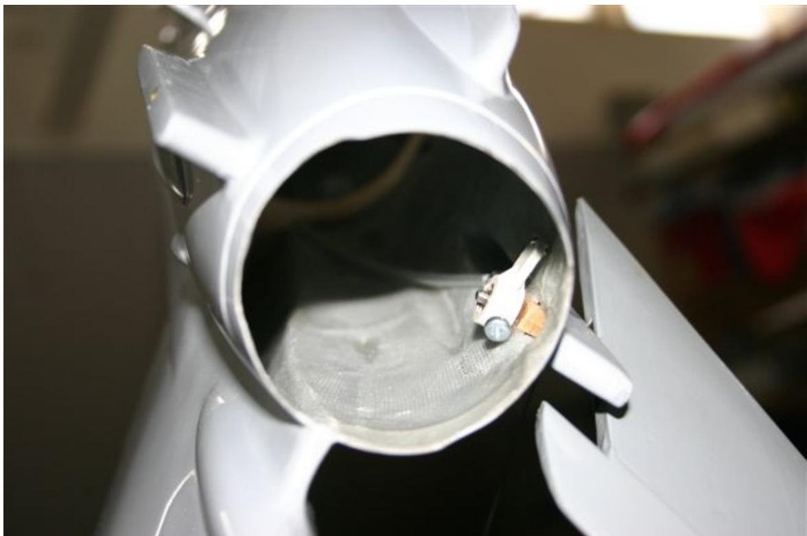
The Bowden tubes are glued on both sides of the fuselages with some tabs of mixed 5 minute epoxy and micro-balloons
