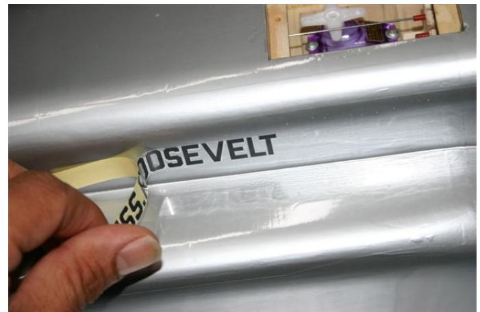
Line out the decal on the area where you want to put the decal. Press the adhesive part. Check if the decal is lined out and remove the rest of the protective back.
