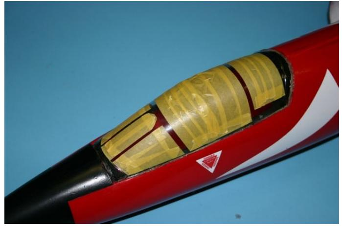
Trim the front, back and bottom edges from the ABS canopy now align it an tape it on the fuselage. Look at the above left picture how the canopy is cut like our mig 29
