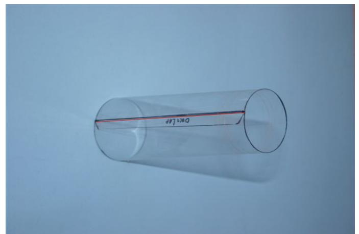
Cut out the unrolled surface for both trust tubes. Put the overlap area inside. Roll the pvc to a tube and apply outside adhesive tape. The Edge should match the innerline of the overlap area. Now you have a perfect conical trust tube.
